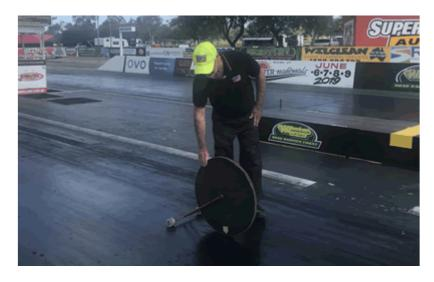
The start line staging beam system has a standard rollout tolerance that needs to be maintained between the Pre-Stage beams, and the Stage and Guard beams. This procedure should be carried out prior to the commencement of an IHRA Australia Event using the 22-inch rollout testing wheel.
