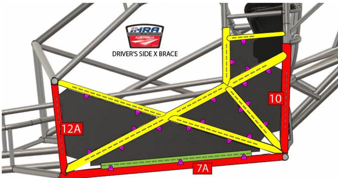
Panels must not be attached to rocker bar (7A), Windshield/Roof bar (12A) or main Hoop (10)
