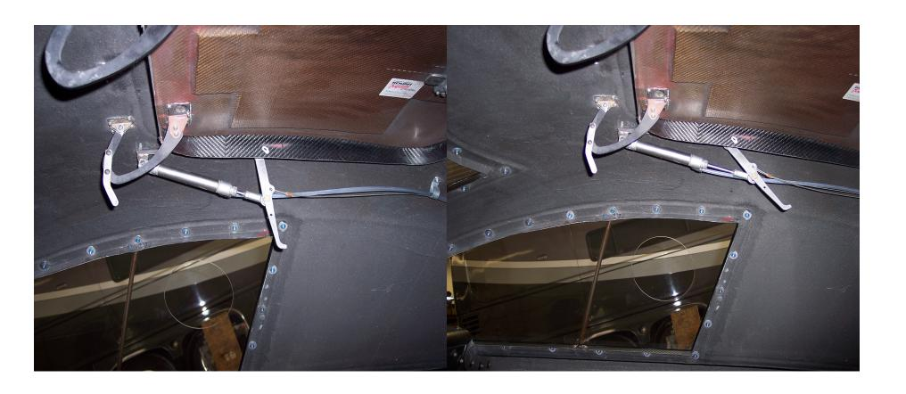
Typical Mounting of Fire Bottle Air Switch.
