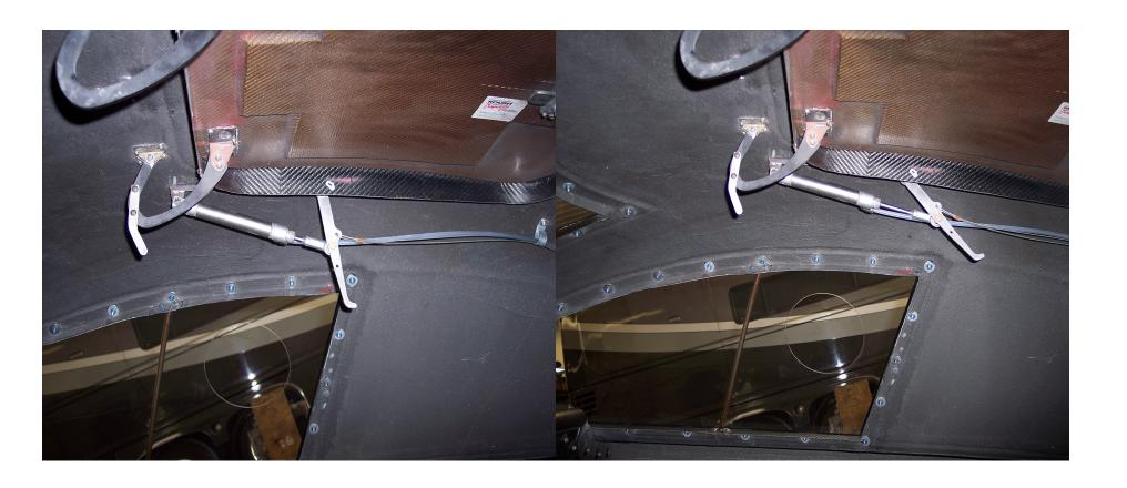
Typical Mounting of Fire Bottle Air Switch.
