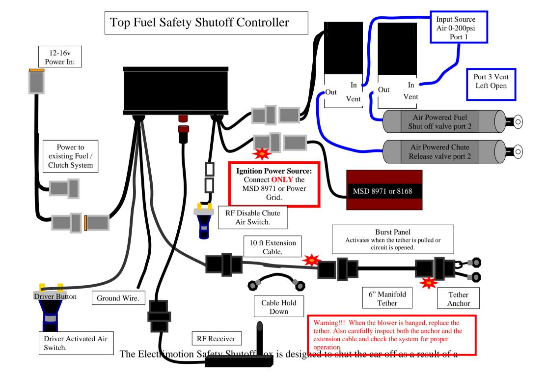
catastrophic event. The box has 3 trigger inputs, which will trigger 3 separate output events. The 3 trigger inputs are a burst panel input, an air activated driver push button trigger input and a wireless shut down input.
